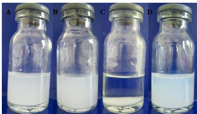
Fig. 4. Dispersion of SNC in water: intact SNC (A); cross-linked SNC with 6% SHMP (B), intact SNC, 0.5 h later (C) and cross-linked SNC with 6% SHMP, 72 h later (D).
